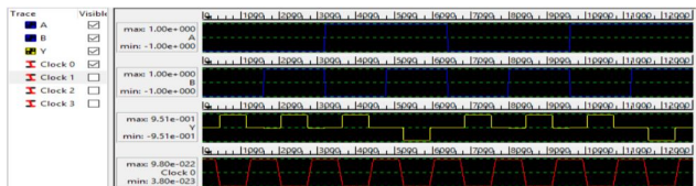
Fig. 16. Simulation Of QCA NAND Gate
